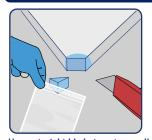
Use a straight blade to cut a small sample. Do not use a serrated edge or disturb the material any more than is needed.
