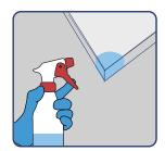
Fill a spray bottle and use a fine mist to wet the sample in order to reduce airborne fiber release.
