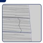
For FIBER CEMENT SHEETING, take the sample from a corner edge or along an existing hole or crack
