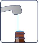
Turn the water to a low flow and fill both bottles completely, leaving a slight meniscus of water above the top lip.
